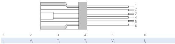
I: applied current V: measured voltage T: temperature sensor
