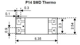
Please consider position and size of the SMD soldering pads on the PCB to be similar to the rectangular part outside of the connecting pads on the chip.
