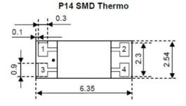
Please consider position and size of the SMD soldering pads on the PCB to be similar to the rectangular part outside of the connecting pads on the chip.
